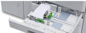
**High Capacity Tandem Tray Configuration** holds a total paper capacity of up to 3,140 sheets.
